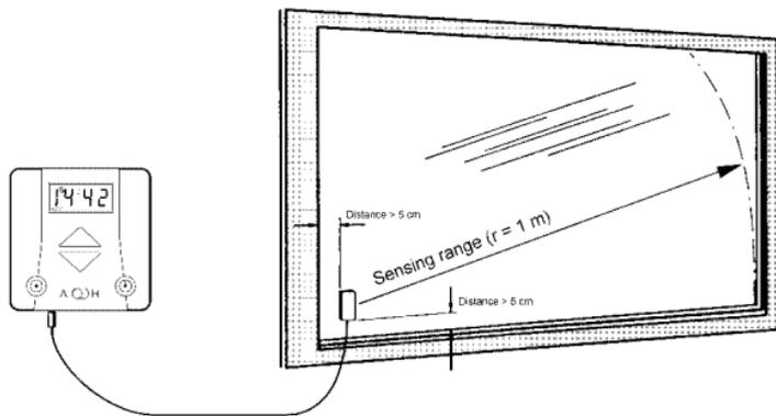
The additional function "broken glass indicator" requires an extra broken glass indicator for each **Vestamatic Rolltec Plus G/S 500** (for larger or separated window panes). The installation of the sun sensor is described below.
